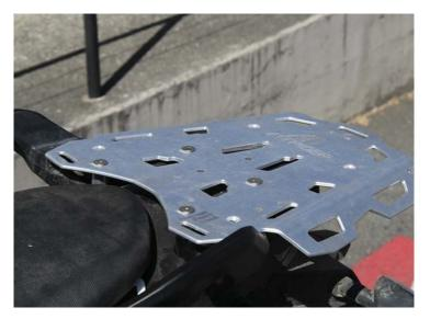
Repeat steps 2 and 3 with the next grab handle. Once all (4) bolts are in place loosely, check the angled spacer alignment and turn by hand to the correct position if needed. Torque the bolts to 15 nm.
