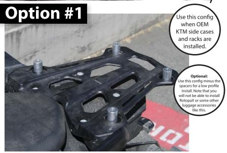
Option #1, install AltRider rack directly on top of OEM rack. First place the (4) 22.2mm spacers in the (4) small indentations on the OEM rack.
