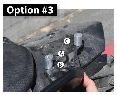
① DSUJ i [fZ YcST ZS` V ₩ Front is a stack of 22mm straight spacer (A) plus 8mm angled spacer.(B)
