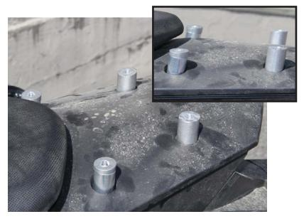
Place the AltRider provided space combo as shown with 8mm angled spacers stacked on top of 22.2 mm spacers closest to the seat, and 25mm sloped spacers nearest the back of the tail. Low point of the spacer should face forward (towards the seat).
