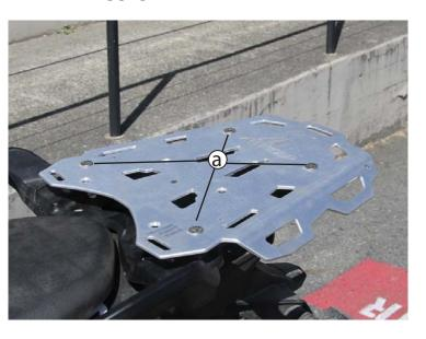
Place the AltRider rear rack on top of the spacers and insert the Two(2) M8 x 45mm bolts and two(2) M8 x 50mm bolts. Use thread locker, and tighten in alternating pattern to 15nM.
