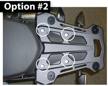
① Option #2, install rack with no OEM rack or grab handles. Remove the OEM rack and grab handles by using a T40 driver to remove the (4) OEM bolts.
