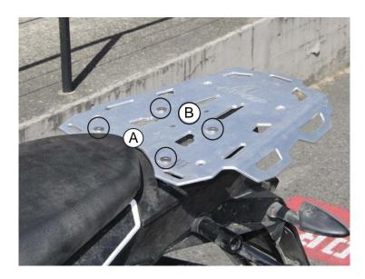
Place the AltRider rack over the spacers. Use thread locker. Insert the two(2) M8 x 50mm bolts in the front holes (A). Insert the two(2) M8 x 45mm bolts in the rear two holes(B). Torque to 15 Nm.
